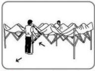
Note: For 20' x 10' tent each person should move to middle leg of 20ft side. Grasp bottom of the tent, lift up and step backwards at the same time until tent is fully opened.
