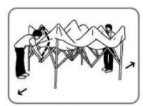
Grasp at the bottom of the canopy tent on opposite sides, as shown. Lift up and step backwards until tent is fully opened.
