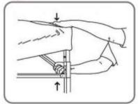
Engage the push button at each corner by pushing up with one hand while holding down top of leg with the other hand. Push button will engage in the hole by locking in.
