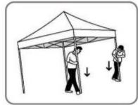
Lift two adjacent outer legs up and pull out the inner legs until snap locks. Repeat on all legs. Raise or level the tent using push button found near bottom of each
